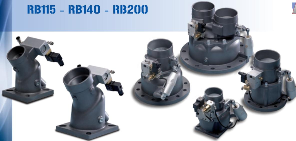
**APPLICATION:** Installed at the compressor inlet to control compressor capacity. During normal operation the valve open and close in response to a control signal to meet the air demand. Stepless or two point capacity controls are available. At the shut-down a check valve stays closed to prevent back flow through the compressor also if the air flow is interrupted. Many solutions are available for stationary or mobile compressors.
